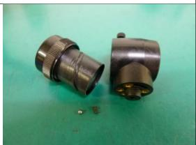
Please rotate and pull the eyepiece part out from the barrel.
