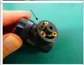
The eyepiece part is fixed on the barrel with a hexagon socket setscrew.
